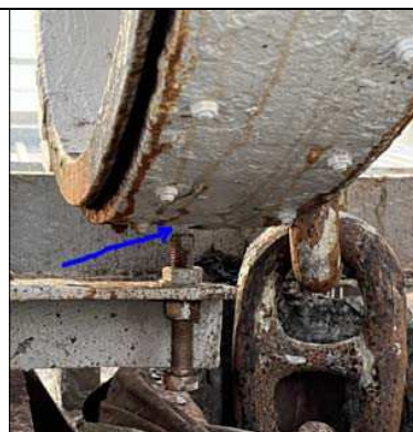
Excessive gap between brake band support screw
